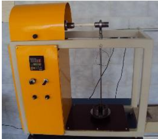
Figure 4. Rotating rock beam fatigue test machine
