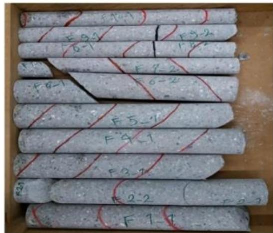
Fig. 9. Procedure for determining the discontinuity surfaces on cores drilled from different concrete blocks.
