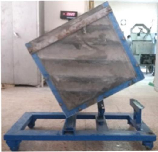
Fig. 6. An overview of preparing physical models with 6-hour intervals to create discontinuity planes.
