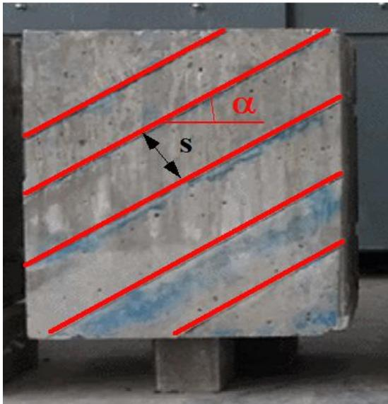
Fig. 7. An overview of concrete block with a discontinuity angle of  $30^\circ$  (Grain size: 0-12.5 mm),  $\alpha$ : the angle between the direction perpendicular to coring/loading direction and the plane of discontinuity, S: spacing of discontinuity planes.
