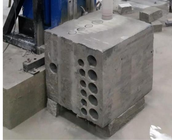
Fig. 8. An overview of drilling in two directions perpendicular to the discontinuity plate.
