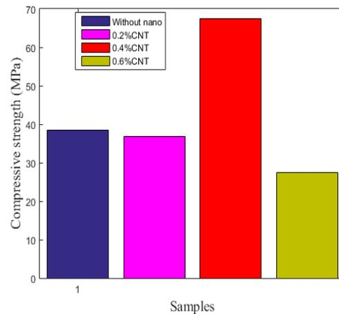
**Figure 5. The compressive strength of samples for pure CNT volume percent**
