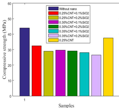
**Figure 4. The compressive strength of samples for low SiO<sub>2</sub> and high CNT volume percent**
