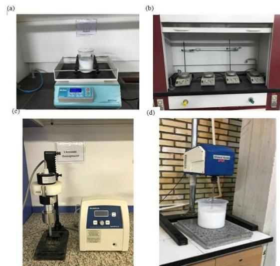
**Figure 1. The procedure of dispersing nanocapsules in water (a) shaker (b) magnetic stirrer (c) ultrasonic devices (d) mechanical mixer.**
