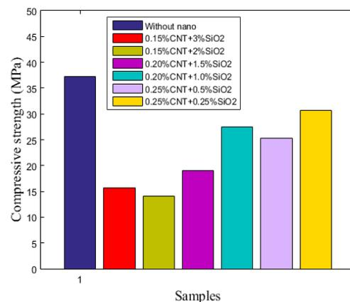
Figure 3. The compressive strength of samples for high SiO<sub>2</sub> and low CNT volume percent
