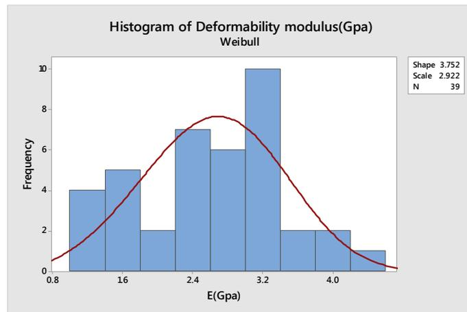
Figure 9. Deformability modulus value distribution
