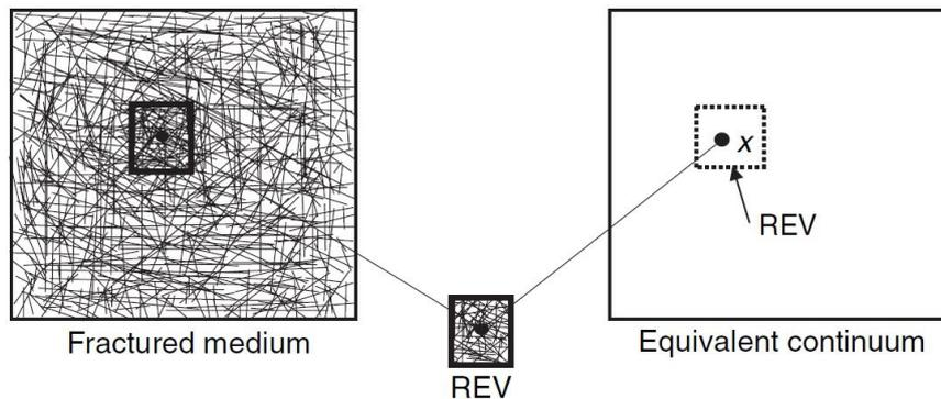
Figure 1. Fractured medium, REV and Equivalent continuum [5]
