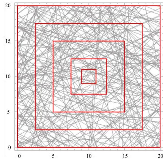
**Figure 5: different model size for a study of the influence of scale on mechanical properties of rock mass**
