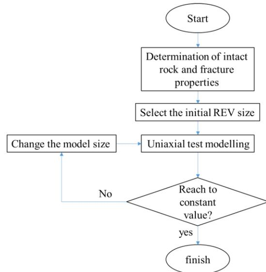
**Figure 4. REV determination flowchart**
