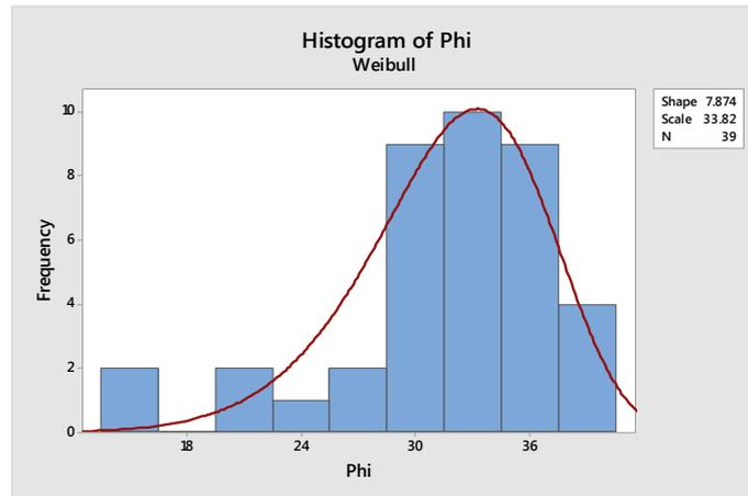
Figure 11. histogram of friction angle
