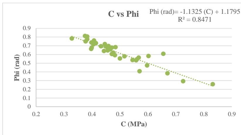
Figure 12: the relationship between cohesion and friction angle
