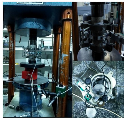
Fig. 5. Uniaxial testing machine with a displacement data logger.
