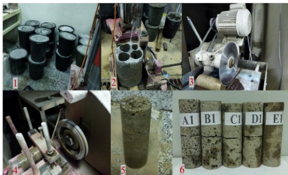
Fig. 4. Sample preparation steps: 1: Preparation of samples with different porosities 2: Preparation of core with standard diameter 3: Cut the sample to the desired dimensions 4: Initial grinding of the sample 5: Final grinding of the sample 6: Sample preparation for testing.
