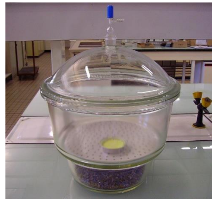
Fig. 2. Desiccator device used for saturation and determination of porosity.
